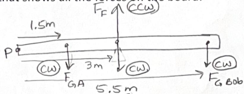
e) If the pivot point for determining the turning ability of the forces is now chosen to be at the left end of the board, label each force on the FBD with the direction of its turning ability as none, CW, or CCW.
