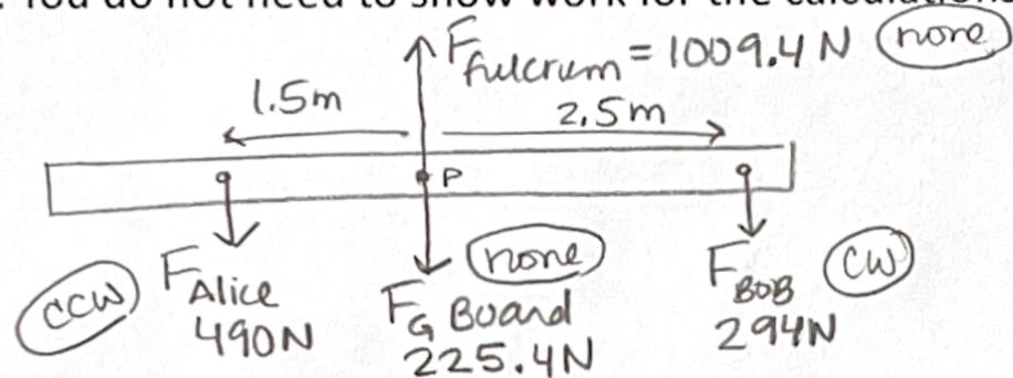
c) If the pivot point for determining the turning ability of the forces is chosen to be **at the fulcrum**, label each force on the FBD with the direction of its turning ability as *none*, *CW*, *or CCW*.
