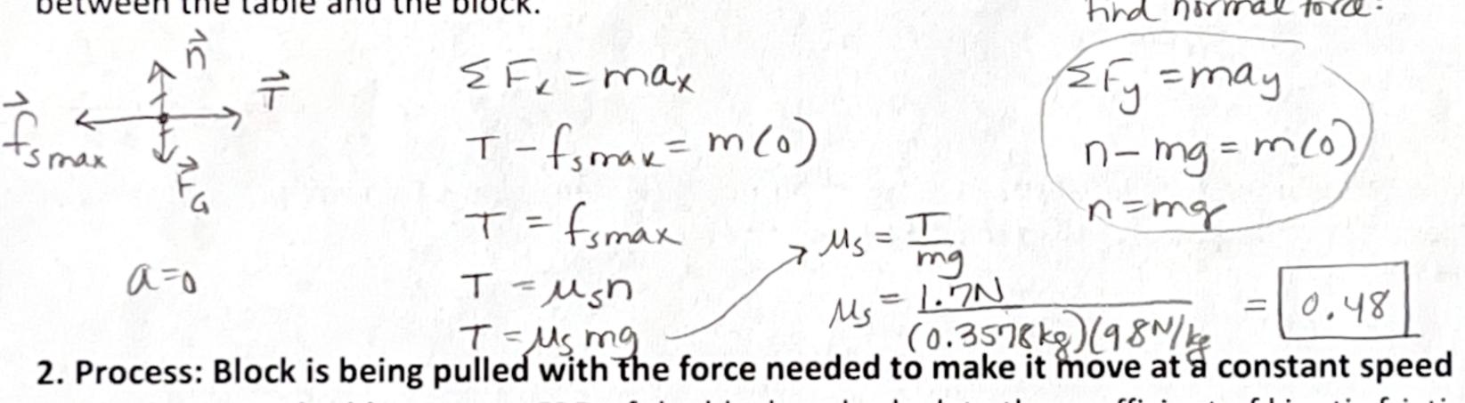
2. Process: Block is being pulled with the force needed to make it move at a constant speed on the horizontal table. Draw a FBD of the block and calculate the coefficient of kinetic friction between the table and the block.
