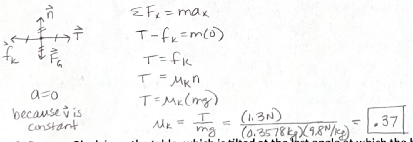
3. Process: Block is on the table, which is tilted at the last angle at which the block will remain at rest. Draw a FBD of the block and calculate the coefficient of static friction between the table
