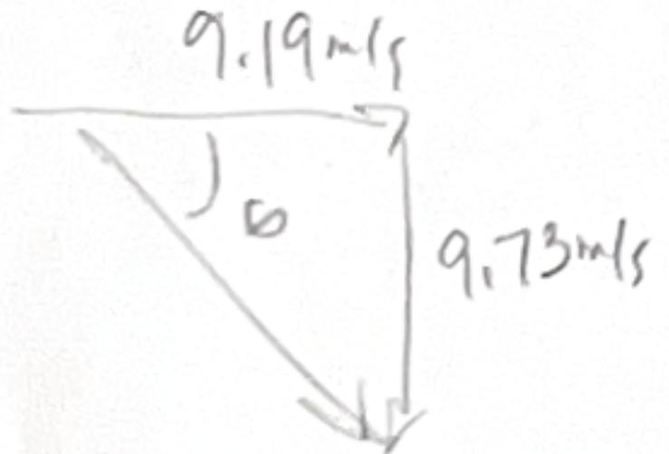
The velocity at impact is 13.4 m/s at  $47^\circ$  below the horizontal.
